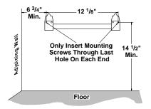
Figure 7 - Mounting Bracket Clearances
